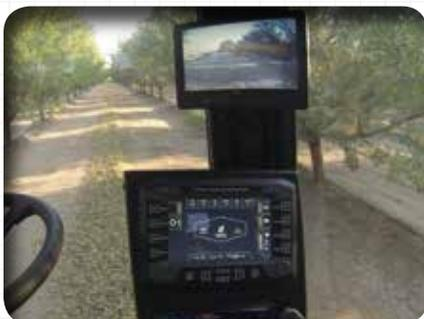
• Rear camera and Plus 1 system for easy operation
