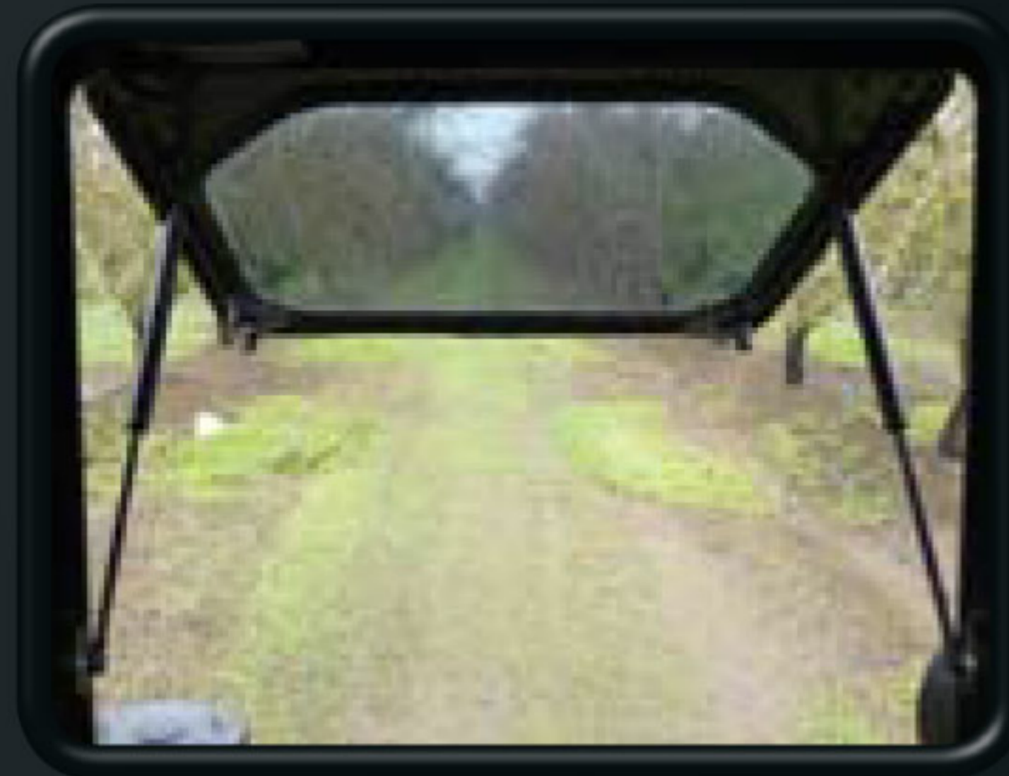
Large hinged rear window equipped with air shock for easy access and visibility during implement hook-up.
