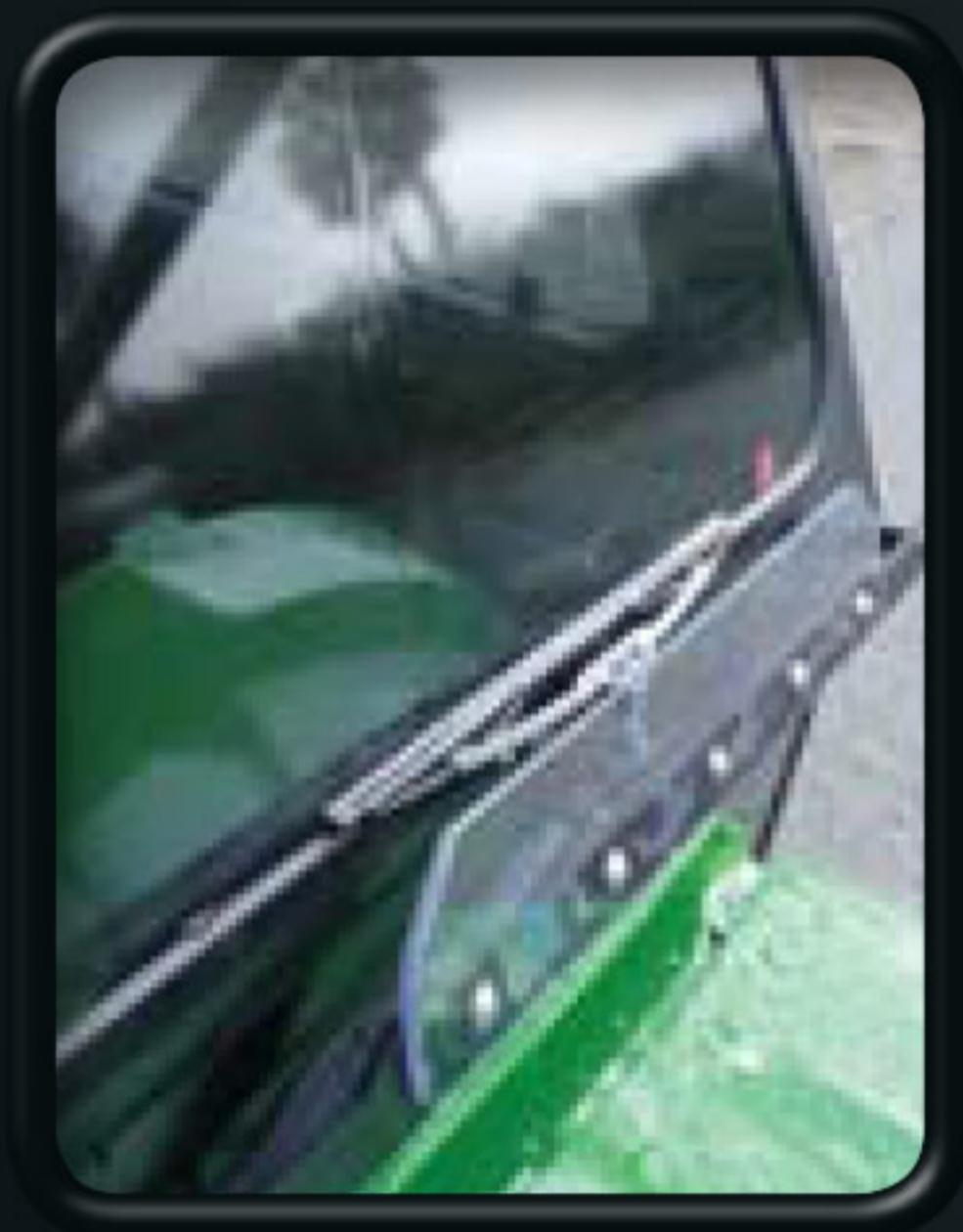
Windshield wiper standard with large wiper fluid reservoir.
